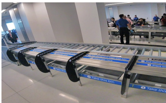
TSA's successful pilot of automated screening lanes includes this automatic bin return system.
