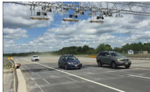
DNDO's Radiation Awareness and Interdiction Network Advanced Technology Demonstration – Monitoring Vehicles at Full Speed for Radiological Threats
