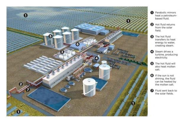
Figure 2-3 Solana Generating Station Diagram
